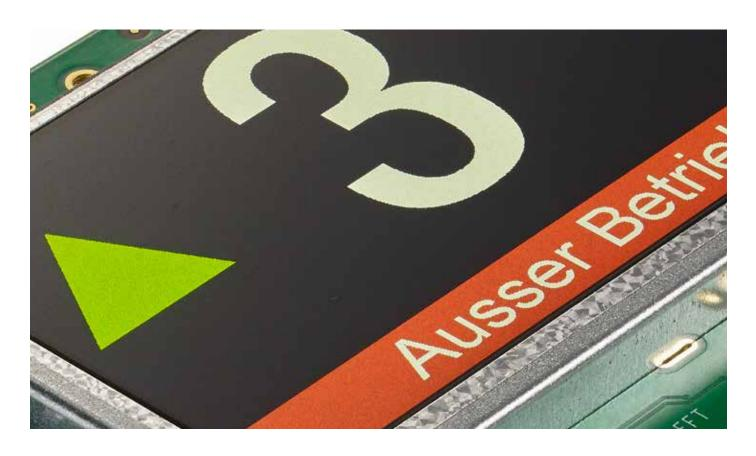
TFT floor display from NEW LIFT
