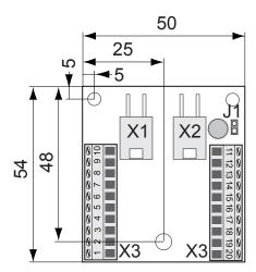
ADM-S and ADM-D circuit board marking
