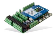
The FST-2XT is designed for use in hydraulic and cable lifts and can handle the different challenges covering the entire range of installations from small to very large.
