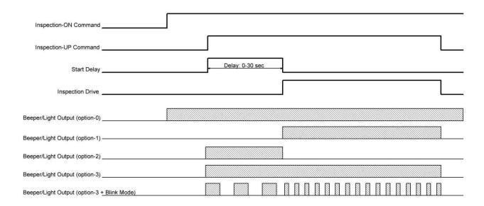
Menu:  $\ \$  Configuration  $\$  Inspection  $\$  Start Delay Up = 0..30 (sec) Menu:  $\$  Configuration  $\$  Inspection  $\$  Start Delay Dn = 0..30 (sec)
