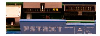
Fig. 2 Jumper is inseted
